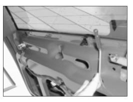
2 Install the repaired panel.
