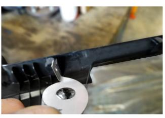
These retaining straps must be angled by approx. 80 degrees, it is best to check the angle by stopping at the panel.
