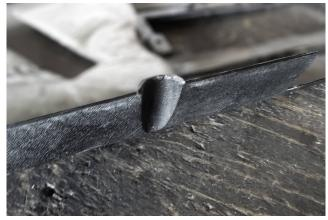
Due to bad treatment or sometimes simply due to brittle plastic, it often looks like that. When individual clips no longer work, the cover does not fall off immediately, but it rattles. The force on the remaining retaining eyelets obviously increases.
