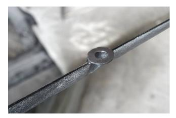
This is how the lower edge of a dismantled tailgate trim should look on a 940. In the centre of the picture, one of the four retaining eyes with which the underside of the trim is attached to the tailgate.
