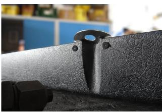
Only then drill the second hole and rivet it. If you drill both holes at once, the sheet metal will almost always be slightly warped after the first rivet and the second hole will no longer fit. It is better, as described, to rivet one side first and then drill the second.
