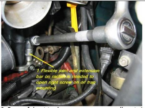
9. Becareful not to drop any screw or small parts in the narrow spaces
