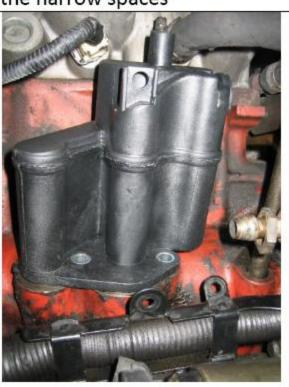
11.Be careful to pull the trap right up, do not shake it if unnecessary, the bottom part may have brittled due to immersed in oil. It will be catasthrophic to break something at this stage, and let it drop into the engine.
