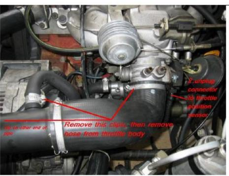
2. This step is the most important because once the throttle inlet hose is removed, the oil trap is visible ans this gives confidence in the following steps.
